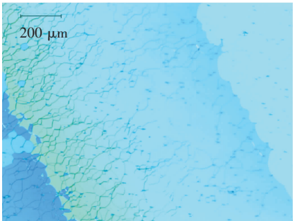
图 5 胆甾相液晶含有畴的平面态偏光显微镜照片 Fig. 5 POM photo of planar state of cholesteric liquid crystal with domain
