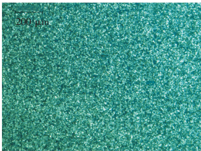
图 4 胆甾相液晶焦锥态偏光显微镜照片 Fig. 4 POM photo of focal conic state of cholesteric liquid crystal
